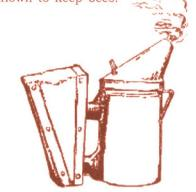
Bottom of smoker gets hot enough to ignite dry grass and leaves. Beekeepers often work in dry grass and leaves. While tin smoker body expands when hot, Niconel "memory metal" top shrinks when heated to make opening and re-fueling nearly impossible.
